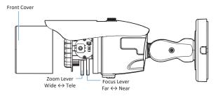
NOTE: If the front cover is cross threaded or not correctly tightened the camera housing will not be weatherproof.
