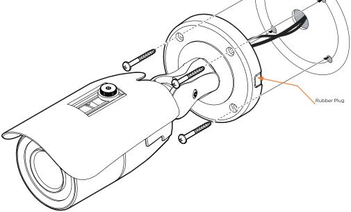
NOTE: Based on the installation environment, remove the rubber plug on the side of the camera's bracket and use the gap as a cable guide to prevent cables from getting caught between the camera and the mounting surface, which can cause damage to the cables and prevent the camera from mounting flush with the mounting surface.
